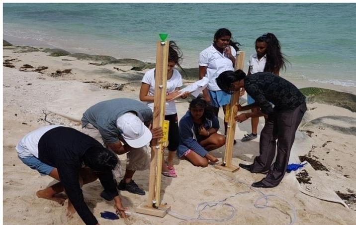
Figure 5: Locally made wooden instrument for beach profiling using the “Emery method”
